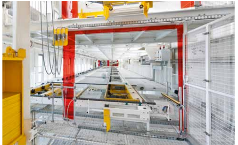
Modern conveying technology: skid conveying stretch with body storage.
